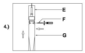
Step 4: Attach glass (G) using set screws (F).
